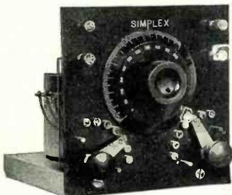
The Simplex Vario-Coupler Panel Mounted makes an ideal short-wave tuner for the beginner, when used in connection with a variometer or variable condenser in the secondary circuit.
