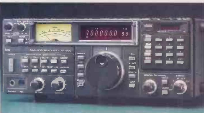
keys to remember. The memories do not store tuning step data, nor the state of the 1GHz button, which is a latching switch for manual use only.
