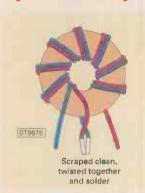
Fig. 1.4: Bifilar winding styles.
