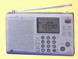
This great new portable has m.w., s.w. and f.m. stereo wavebands and for easy tuning it features direct frequency tuning via the keypad, also auto and memory scanning, which lets you quickly find the station with the best reception. Plus, it has the capacity to store up to 45 stations in its memory. So, wherever you are in the world, you can keep updated on news and music.
