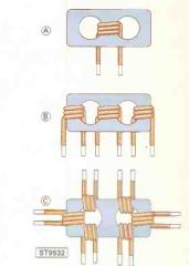
Fig. 3.3: Winding styles for binocular cores (Fig. 3.3a preferred).
