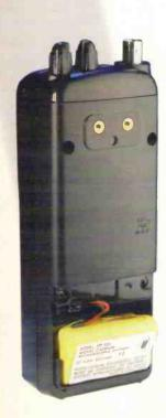
The plug-in heat shrink NiCad battery pack.
