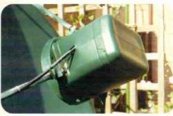
Fig. 2: The 4GHz LNB is protected with this cover made from a two litre polythene white spirit container.
