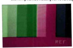
Fig 5: Unidentified 'REF' colour-bar pattern radiated from a UK transmitter. This is probably an internal test pattern which was radiated accidentally.
