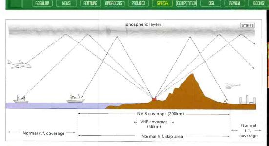
Fig. 1: Near Vertical Incidence Skywave propagation. NVIS bridges the gap between the nominal v.h.f./u.h.f. coverage area and the typical h.f. 'skip zone'.
