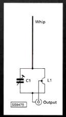
Fig. 1: Circuit of matching transforme
