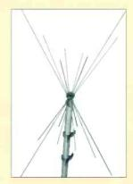
The Airmaster 117-137MHz and 224-400MHz airband antenna is a high performance, dedicated, civil and military airband antenna. Two pairs of angled dipoles cover the 117-137MHz civil band, and six pairs of angled dipoles cover the 224-400MHz military band nominal impedance is  $50\Omega$  via an N-type connector.
