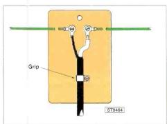
Fig. 6: Dipole connection.
