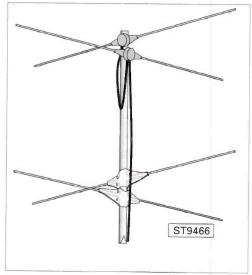
Fig. 8: Standard crossed-dipole.
