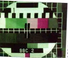
Fig 6: This month's visit to Memory Lane. The BBC-2 Colour Test Card "G" with the countdown clock in the lower righthand comer to indicate the minutes remaining of the Trade Test Transmission. The off-screen photograph was taken in December
