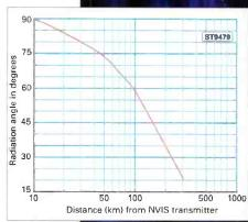
Fig. 2: Graphical representation of the range in km from the NVIS site. yersus elevation angle.
