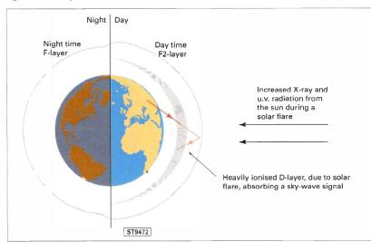
Fig. 6: The cause of a Sudden lonospheric Disturbances (SID).
