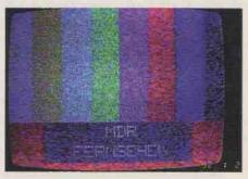
Fig. 2: German FuBK test card from MDR displaying local identification, circa 1992.
