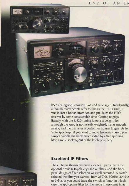
The i.f. filters themselves were excellent, particularly the optional 455kHz 8-pole crystal c.w. filters, and the front panel design of filter selection was well executed. A switch selected the filter you wanted, from 250Hz, 500Hz, 2.4kHz or 6kHz, or you could leave the switch in 'auto' in which case the appropriate filter for the mode in use came in as the receiver mode switch was turned. Concentric with the filter switch was the fully variable bandwidth control, so it
