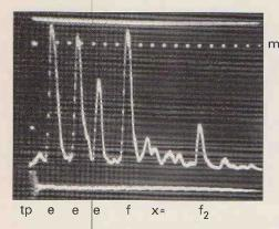
Fig. 2.6: Photo from oscilloscope. Simulation of 'N' mode propagation (tp) transmitted pulse. (e,e,e) pseudo sporadic E primary and two multiple echoes  $\{f, f2\}$  pseudo F region primary and one multiple echo (x) small spurious echoes (see text); (m) Ims: markers.
