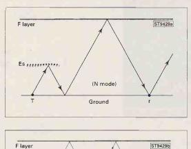
Fig. 2.4: Lonosperic propagation (A) 'N' mode. (B) 'M' mode. Es: Sporadic E cloud (see text).
