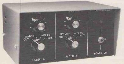
onstruction of the filter is quite straightforward using a piece of Veroboard on which to mount the components and placing the potentiometer and rotary switch on the front panel of a suitable instrument case. The arrangement of the components and the positions where the tracks have to be cut is shown in Fig. 2.1. The layout shown is for two filters, but readers who are interested in constructing only a single filter, should ignore Filter A and start their board at track 13.
