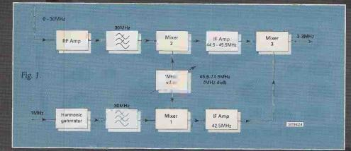
tuneable i.f. preceded by a converter which changes the h.f. spectrum into 1MHz wide 'chunks' to be tuned by the tuneable i.f. The difference comes in that until the introduction of the Wadley loop the front end conversion was carried out by using a crystal controlled converter, which necessitated a crystal for each 1MHz 'chunk' - in fact the method used in the Collins 51S-1
