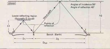
(e) are multiples from a simulated sporadic E cloud (as in **Fig. 2.5**), whilst (f) and (f2) are primary and secondary from the simulated F region (ceiling).
