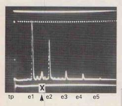
Fig. 2.2: Indoor simulation with ultrasonics of multiple echoes from a psuedo reflecting F region, i.e. the ceiling. Frequency 40kHz; p.r.f. 20Hz; pulse width 1ms; Markers (m) 1ms; (tp) transmitted pulses; (e1) primary echo; (e2, e3, e4, e5) multiple echoes; (x) see text.
