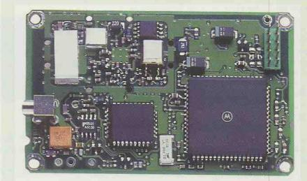
New features on the UT Plus Oncore GPS from Motorola give the receiver greater immunity from unintentional jamming.
