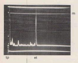
Fig. 2.9: Photo from oscilloscope. Simulation of OTH radar. (tp) transmitter pulse; (et) echo from target located near earth (bench) at a surface distance of 2.24m; (m) 1ms markers (see text).
