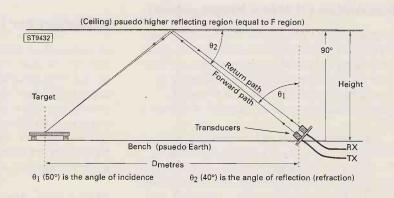
Fig. 2.8: Arrangement for simulation of Over The Horizon Radar (OTHR).
