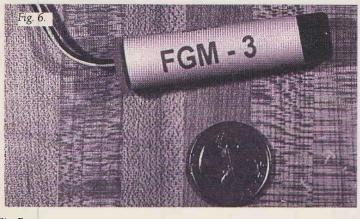
Fig. 7. Red -0 +5V d.c. White FGM-3 O Signal out Black Gnd. FGM-1 3 1 - Feedback ST9402 2 - Signal out 3 - Gnd. +5V d.c. Fig. 8. 24 22 20 18 16 (STI) 14 12 10 8 6 -0.8 -0.6 -0.4 -0.2 0 +0.2 +0.4 +0.6 +0.8 H (Oersted) ST9403
