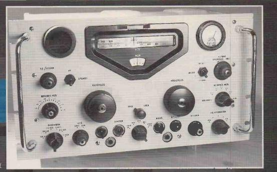
signal from the high frequency 'MHz' oscillator is also fed to a second mixer, the output of which is taken to a band pass filter and i.f. amplifier covering the range 44.5 to
