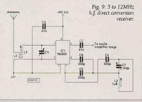
example, the value of inductor L3 can be changed to a higher or lower value for tuning to another frequency.
