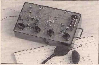
The manual contains complete schematics and theory of operation of all the building blocks. Use this trainer to receive frequencies from 500kHz to 110MHz!
