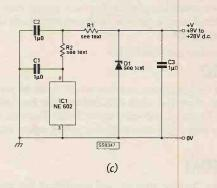
Fig. 3: The d.c. power supply connections for the NE602.
