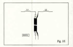
Fig. 8: Modified Windom with 4:1 BALUN to transform impedance and coaxial cable feedline.
