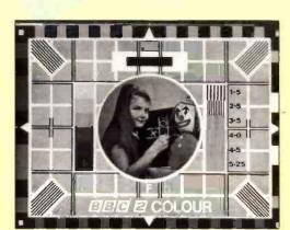
Fig. 2.4: The original version of the BBC Colour Test Card 'F' transmitted from 1 July 1967.
