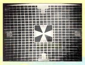
Fig. 2.1: This monochrome Test Chart was used by the BBC in the fifties to check colour camera registration.
