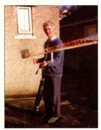
Fig. 2: Yagi for METEOSAT WEFAX reception.
