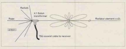
Fig. 1: The basic resonant (unterminated) long-wire antenna.
