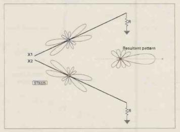
Fig. 5: The non-resonant Vee-beam antenna.
