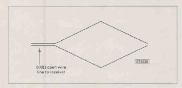
Fig. 8 Resonant rhombic antenna.
