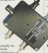
construction of the T2FD antenna. A specially wound 9:1 Balun, together with a thick film  $500\Omega$  5W termination resistor, is fitted into a small ABS box. The completed assembly is encapsulated in epoxy resin to ensure reliability in the most severe weather conditions.
