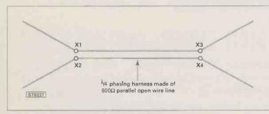
Fig. 7 Stacking Vee-beams gives 3dB more gain.
