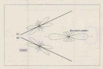
Fig. 4: The basic resonant Vee-beam antenna.
