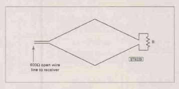
Fig. 9 Non-resonant rhombic antenna.
