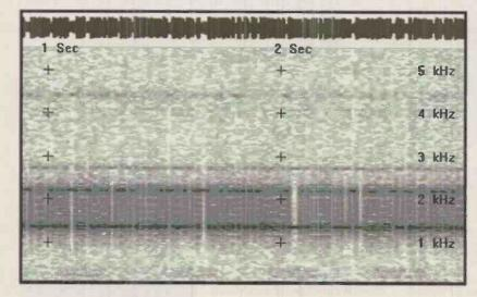
Fig. 2: Spectral display of part of the signal in Fig. 1. The display was obtained with an FFT (Fast Fourier Transformation) program sampling at 512 points at a sample rate of 11.025kHz.
