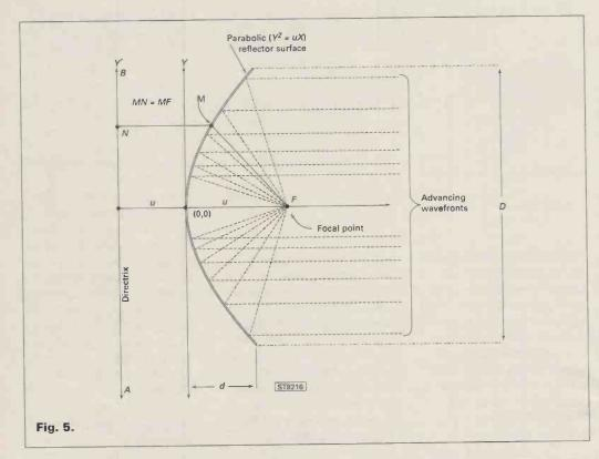
The gain of the parabolic dish antenna is found from:
