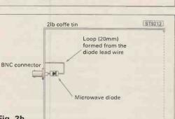
solution was to use the 'coffee tin antenna' of Fig. 2b. This antenna is related to the cavity style, but it uses a discarded metal coffee tin as the cavity. We found that the two pound American size tin gave around 6dB gain for little effort, as nearly as we could measure it.
