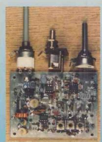
The Hands **Electronic RX1** superhet receiver. This is the completed printed circuit board awaiting testing and alignment before being fitted into a The RX ! p.c.b is quite densly packed and needs a steady
