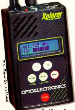
•Two-Line LCD display, first line displays frequency. Second line switches between either CTCSS, DCS, DTMF, Signal Strength, or Numerical Deviation.
