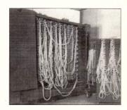
Rear view of British 3-rotor Bombe, showing wiring of plugboard for daily changing.
