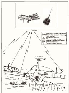
Fig.2: Basic Concept of the COSPAS-SARSAT System. Courtesy of IMO
