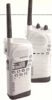
Pic 4 Two typical GMDSS v.h.f. hand-helds from Navico. Courtesy of Navico Ltd.
