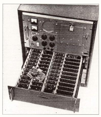
Open resonator tray showing the 33 tuned circuits, one for each of the tones in the three rows of slots on the left.
