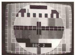
Fig. 6: A PM5544 variation, known as Test Card 'G', as used by BBC-1 and BBC-2 during the Seventies and Eigthies, mainly for regional opt-outs.
