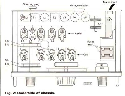
The rear panel of the set houses the voltage selector, the set will operate from 100 to 125V or 195 to 250V a.c. or d.c. Also on the rear panel are the two antenna sockets and the earth socket.
