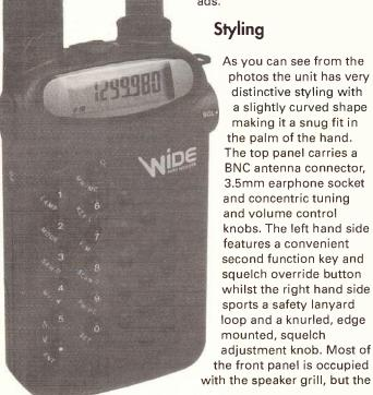
rotary control can be used to manually tune up and down in frequency at a rate determined by the preset step size. This can be set to be either 1, 5, 6.25, 9, 10, 12.5, 15, 20, 25, 30, 50, 100kHz or Automatic - but more of this later.
