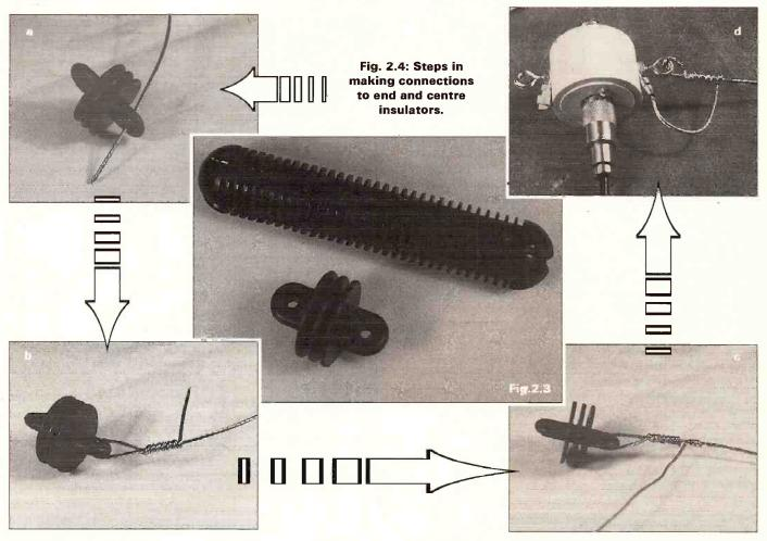
electrical connection. The solder is needed, but keep in mind that most of the electrical connection and all of the mechanical connection is provided by a good, tight wrap, not by solder.
