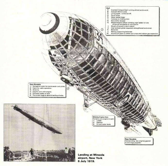
The end-fed long wire was on a drum with a handle attached to it and when needed the handle was turned so that the antenna would hang down vertically for about 91m from the forward control cabin and operated on a frequency of 230kHz - now a part of the long wave band.
