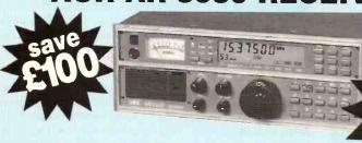
30kHz-30MHz AM, SAM, SSB, CW, FM 100 memory channels
