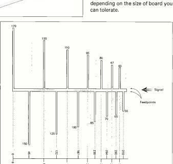
Fig. 3: The basic dimensions of the elements.
