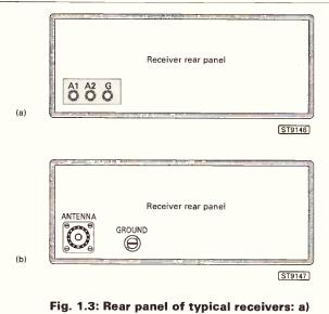
screw-terminal type; b) coaxial cable type.
