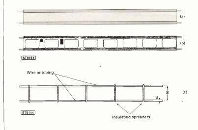
Fig. 1.1: a). 300  $\Omega$  twin-lead; b). 450  $\Omega$  twin-lead; c). parallel open line.
