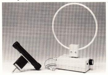
The aerial elements may be rotated in order to achieve maximum receive signal strength while minimising (nulling out) the effects of unwanted interfering local terrestrial signals. The vari-cap tuning featured in the LA320 also adds valuable selectivity to any receiver's front-end stages.
