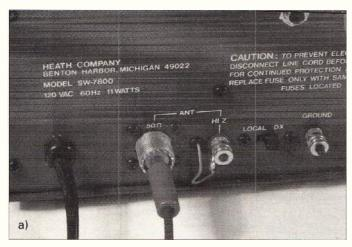
Fig. 1.7: a) Connecting a single-wire downlead to a coaxial connector; b) Connecting a single wire to a coaxial cable not recommended, but it works.
