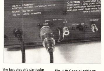
Fig. 1.8: Coaxial cable to coaxial connector.
