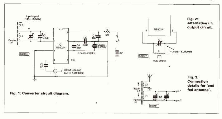
quite simple circuitry with a few external components. The pin configuration of the NE602N is shown in the circuit diagram **Fig. 1**.
