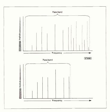
Fig. 1.1: The interference on the signal in (a) is removed by the reduced bandwidth in (b).
