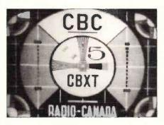
A distinctive test card used until the early seventies by Canadian TV. The callsign and channel number were included in the centre. This example was radiated in the Edmonton area. The transmitter had an e.r.p. of 318kW.
