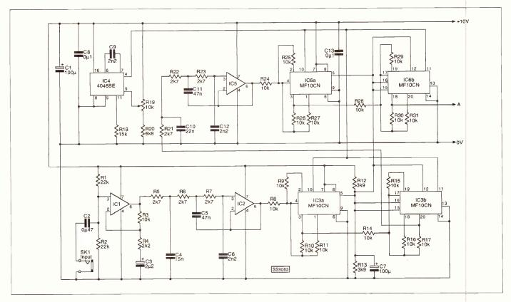
other sections of IC4. Capacitor C9 and R18 are the timing components, and a variable control voltage is provided by R19 and R20. Resistor R19 provides an operating frequency range of about 20kHz to 55kHz. IC5 is used in a third order low-pass filter connected between stages two and three of the high-pass filter.
