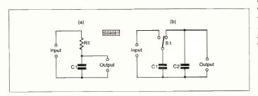
Fig. 1.2: (a) A conventional CR low-pass filter and (b) a switched capacitor low-pass filter.
