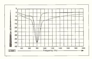
Fig. 1.8: The notch filter responses with high and low Q settings and an 800Hz centre frequency.
