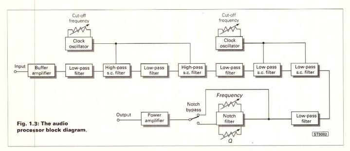
main purpose. It ensures that any high frequency components on the input signal are not allowed to pass through to the switched capacitor filters where they could heterodyne with the clock signal to produce audio tones at the output.
