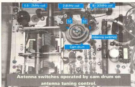
Fig 1: The cam and switches used in the r.f. stage
