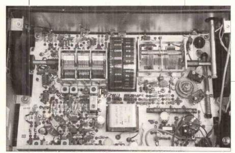
Inside the XCR-30, r.f. tuning on the right, v.f.o./mixer/i.f. tuning on the left, a.f. output bottom right. The batteries are carried in a holder on the back cover (lifted away in this shot).
