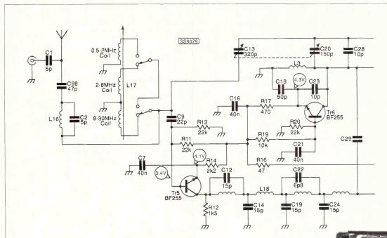
Fig 3: A portion of the circuit diagram showing the antenna switch details.
