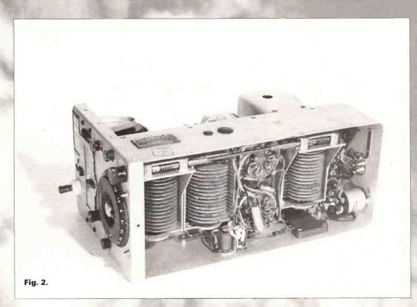
Command transmitter BC-458-A underside view showing the ganged v.f.o. and p.a. tuning mechanism.
