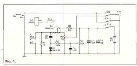
When switched 'On', the loop or bandpass filter is enabled (depending on whether or not the loop is plugged in), the wire antenna at SK1 is earthed to avoid spurious pick-up, and power is applied to the circuit. When 'Off', S1a and S1b connected the wire antenna straight through to the receiver and disables the loop/bandpass filter.
