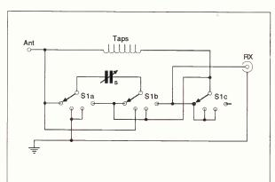
Fig. 2: Circuit diagram of the modifications needed to switch the four types of a.t.u.
