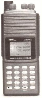
The AR8000 UK receiver is without doubt the most full featured wide band hand held receiver on the market today. Frequency coverage is from 500 kHz - 1900 MHz without gaps with all mode reception... twin frequency display, alphanumeric text comments. AR8000 £449 UK carriage free SC8000 case £17.95 + £1.50 P&P CU8232 interface £99 + £3 P&P PC-MANAGER DOS software £49 + £3 P&P
