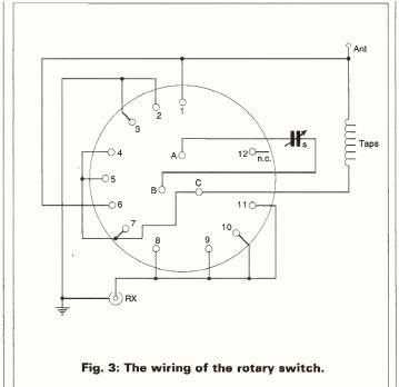
to be made in the back of the case to mount the switch, care being taken not to damage either the coil or the original 12-way tapping switch and its wiring. Wire the new switch with all connecting leads before mounting it on the back panel. Then 'dress' the new wires to give short, neat connections.
