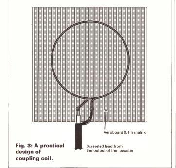
shows how. Probably the most practical design of coil is that shown in **Fig. 3**. The coil consists of about ten turns of enamelled copper wire (30s.w.g. will do again) supported on a 40 x 40mm piece of Veroboard. The screened lead feeding this coil need not be 'proper' coaxial cable, microphone lead being perfectly good enough and more flexible. The coil can be glued to the board, or if you have the facilities it could be
