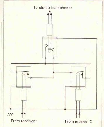
Fig. 1: The circuit of the Two-Hooks ensemble.
