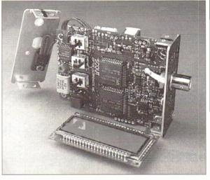
frequency measurements are made continuously. Captured frequencies are displayed on the l.c.d. display. On capture of a new frequency one of two warning devices are activated, either the beeper, or for a more discrete warning the vibrator. If the beep is selected then the display backlight is also illuminated for ten seconds.
