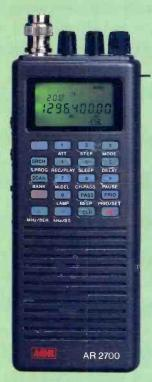
The NEW AR2700 UK receiver is the very latest high-tech hand held receiver from AOR. Frequency coverage is 500 kHz - 1300 MHz with receive modes of NFM, WFM & AM. A large LCD with three way rear illumination provides all operational details. An optional VOICE **RECORD** chip RU2700 permits an instant 20s digital recording off air which may be replayed over
