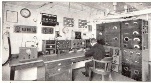
Typical 1930s Marconi passenger ship installation showing 2kW CW/ICW long wave transmitter type 388/387/389 and antenna distribution switches. On the desk can be seen 250W QG emergency transmitter and type 352A and 521 receivers. The receiver on the extreme left is used for broadcast reception.
