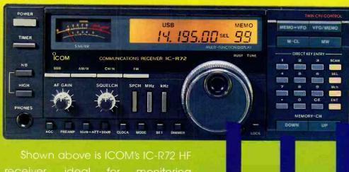
Shown above is ICOM's IC-R72 HF receiver, ideal for monitoring broadcasts, marine vessels, aircraft and emergency services on AM, SSB, CW plus optional FM between 100kHz and 30MHz. The IC-R72 has high sensitivity, an advanced DDS system, 100dB dynamic range and a very interesting range of options, as does the IC-R7100...
