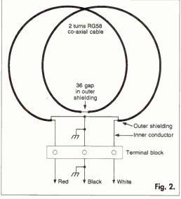
hielded loop antennas take the form of a nonmagnetic metal tube enclosing the loop conductor winding. This shield must not form a continuous electrical path, so a small gap in the shield is usually made opposite the feed point, as shown in Fig. 1.
