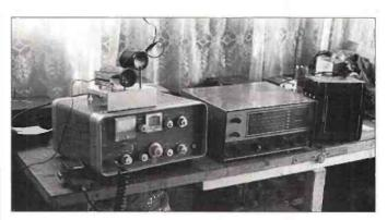
Using the Heathkit RA-1 with a KW Vespa as an amateur station.
