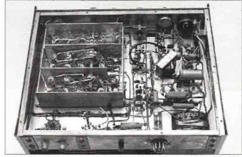
Internal view of the Heathkit RA-1, 6-band coil pack on left
