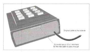
Fig. 6: The end of the kepyad showing where to file the small notch needed to allow the ribbon cable to exit the box.
