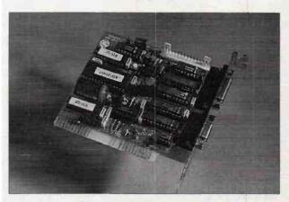
Sonifex announce their new Mentor MSF radio clock system, designed to ensure that your PC is synchonised to UK time automatically by utilising the broadcasts from the 60kHz l.w. Rugby MSF station. The signal from Rugby can be received in most UK locations.
