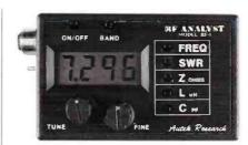
microprocessor, A/D converters and a low-distortion, levelled, sine-wave generator with a 4-digit frequency readout, continuously adjustable from 1.2 to 35MHz in five bands. It measures r.f. values of impedance (0-2000 $\Omega$ ), s.w.r. (1 to 15:1), Capacitance (0-9999pF) and Inductance (<0.04 to 300µH). The digital readout of all parameters is claimed to be unique in its price range.
