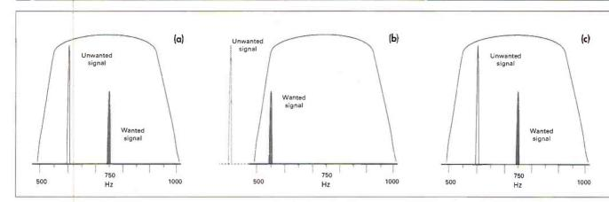
Fig. 4: (a) A typical situation where a wanted c.w. signal is overshadowed by a stronger one and both signals are in the pass-band of the filter.(b) shows how the unwanted signal may be dropped of the lower edge of the filter by re-tuning the receiver. This does change the received c.w. note. c and d shows how an i.f. shift control may be used to isolate the wanted signal, leaving the c.w. note the same.
