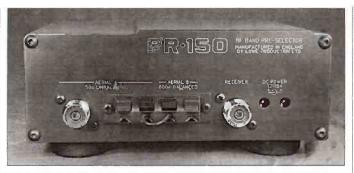
Versitile antenna connectors and power out socket make this an extremely good mate for the Lowe Electronics HF-150 communications receiver.
