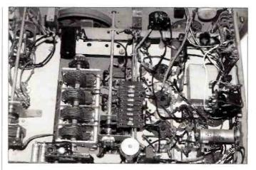
ensure earth continuity. Mains voltage creepage distances were checked by measuring between all live connections and associated components and was found to be over 3mm, as required by today's standards. The mains input to the power supply was switched and then fed back out to the receiver 230V a.c. connection.
