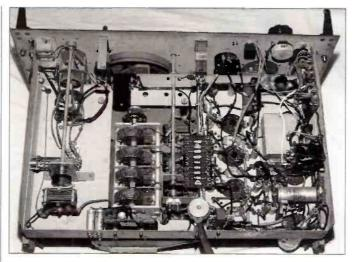
Two views of the underside of the B21B's chassis. The construction is typical of sets of this period.
