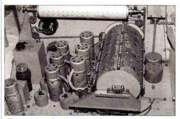
Close-up view of the band selection drum, operated by the large T-handle on the front panel.
