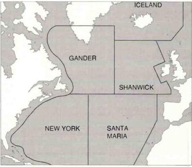
Fig. 1: The North Atlantic is split into five areas for h.f. aircraft communications.
