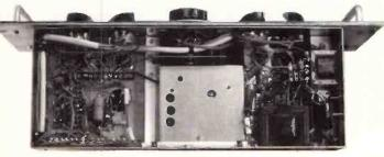
Top Internal View: Shows RF-Mixer-Oscillator unit built in a separate box with the twin antenna filter mounted near back edge. The divide by 100 module can be seen attached to the back of the frequency display unit. The relay at the right was added after the article was written and is for the control of the tape recorder.
