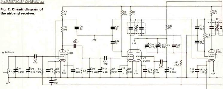
be varied to get the required oscillator coverage. It is a good idea to make this capacitor variable to enable the frequency coverage to be adjusted. I used a Philips 3-30pF trimmer and this proved to be ideal but it may require a fixed capacitor across it to get the desired tuning range.
