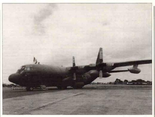
KCC-130 Hercules refuelling tanker, it weighs 82921lbs dry!
