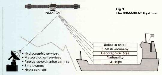
and alert land stations, including rescue co-ordination centres, and pass on the distress to other vessels in the area. Separate systems aboard the ship will allow her to communicate with other vessels as well, in effect doubling the transmission spread.
