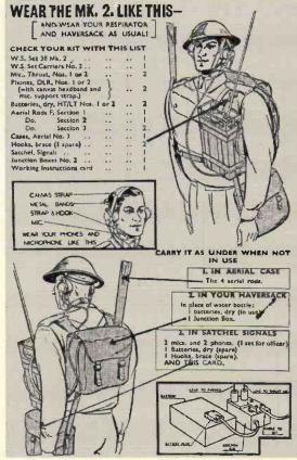
Fig. 1: An instruction sheet on how to wear the No. 38 set.
