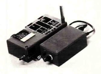
The 328R receiver and its new battery pack.
