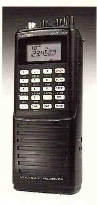
features which impressed me initially. There is a small button on the side panel labelled **LAMP**, which (when pressed) provides a backlight to the liquid crystal display and also all the keys on the front panel. The previous model from Yupiteru (the MVT-7000) only has a light for the liquid crystal display, so seeing the keys light-up was particularly impressive. The light stays on for as long as the button is pressed, so that there is only minimal power drawn from the batteries.
