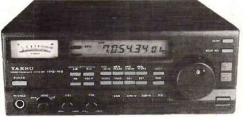
coming and the FRG100 sets a new standard from this manufacturer. Broadcast listeners may like the 6 and 4kHz bandwidths and the fifty memory channels will store both frequency and mode.
