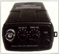
scanning function is the ability to scan only those memory channels that contain the same mode (i.e., a.m., f.m., etc.) as the mode at the start of the scan. This came in handy when I wanted to scan only the f.m. frequencies at my local airport; it means that you don't have to go through all the memories **PASS**ing all the frequencies that are not in the mode that you want to scan in.
