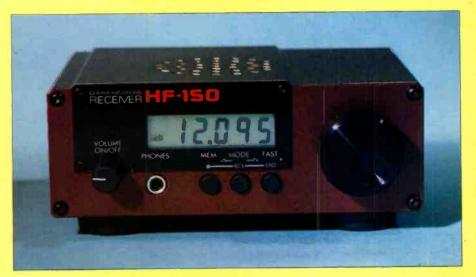
Aerial inputs: 600 ohms, 50 ohms & Hi-Z Whip Power: 12Vdc from mains adaptor (supplied) Case: All-metal light alloy case Size: 185mm(W) x 80mm(H) x 160mm(D) Weight: 1.3kg (less batteries)
