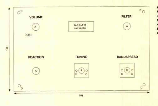
Fig. 2.3: Front panel layout of the receiver. Hole sizes. A=10mm; B=8mm; C=2.5mm on 14mm centres; D=3.5mm.
