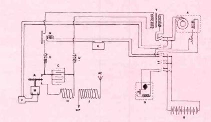
Fig. 2: The transmitter circuit. (A) 60Hz Alternator. (B) 110V storage battery, (C) High tension condensor, (G) 110V battery charging generator, (H)
