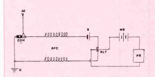
Fig. 3: The receiver circuit. (AE) Connection to main antenna, (B) Coherer battery, (COH) Coherer detector, (MB) Receiver battery, (PR) Morse printer, (RFC) RF chokes, (RLY) Relay.
