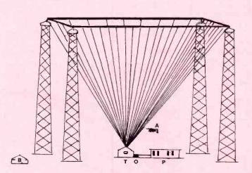
Fig. 1: The South Wellfleet transmitter site. (A) The main antenna assembly; (B) Personnel living quarters; (T) The transmitter house; (O) Wireless operator's hut; (P) Transmitter power house.
