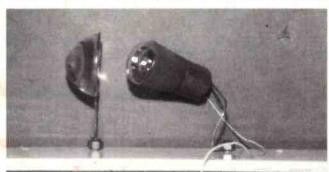
The neon indicator light source in the typical bullseye lens.
