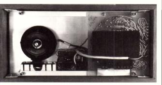
The Indicating Unit with the back removed. The battery is in the bottom left.
