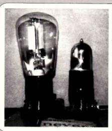
Magenta AC/HL valve (left) and a Cossor triode type D336 or similar. sound. A separate receiver was, of course, necessary for the reception of the sound channel. Both stations gave good reception at our home in Rotherham.
