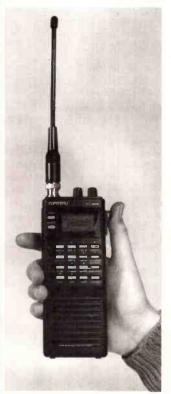
The VT-225 is a civil and military airband receiver, covering 108-142MHz v.h.f. and 222-391MHz u.h.f. Its main features are:
