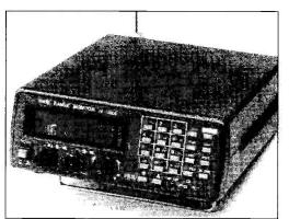
AR2800 Base/mobile scanning receiver. The frequency coverage is 500kHz – 600MHz and 800MHz – 1300MHz. All mode AM, FM (narrow), FM (wide), and built-in BFO for USB, LSB, CW. The AR2800 features 1000 memories for spot frequencies and 10 search banks. Operation of the receiver is fairly easy and is similar to that of the popular AR1000/AR2000. The AR2800 is operated from 13.8V DC and is supplied with an AC adaptor, DC lead, mobile mount and telescopic aerial.
