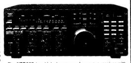
The NRD525 is a high-class, general coverage received expandability looking to the future. combining traditional technology unique to JRC with the most advanced digital technology gives superb performance whilst remaining extremely easy to use. The NRD525 covers 90kHz-34MHz and with an optional VHF/ UHF converter also covers 34-60, 114-174 and 423-456MHz. Modes of operation CW, SSB (USB/LSB), AM, FM and RTTY with optional
