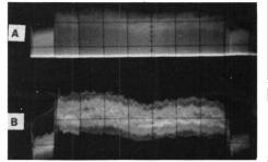
Fig. 5: Signals that appear around 20MHz and which 'sound' like those from a Russian 'Woodpecker' transmitter. (A) Carrier with negativegoing pulse modulation (nP). (B) Rectified signals plus noise (see text).
