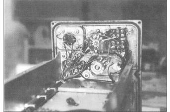
The inside of the R210 showing the back of the front panel with the new Octal socket and its wiring.
