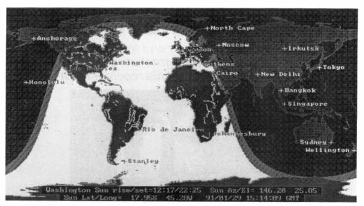
Printout of file GEOCLOCK02.PCX showing the daylight areas of the earth's surface and the Greyline, at a lower resolution than the previous printout.
