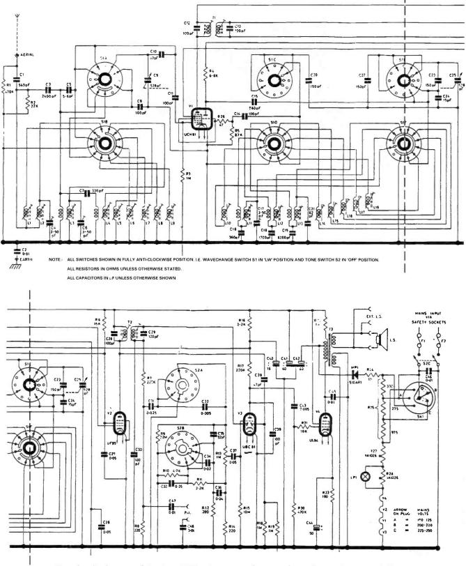
The circuit diagram of the Pye 3017A (Export) radio taken from the service manual. The diagram has been split into two, about the vertical broken lines, to enable it to be fitted onto this page.
