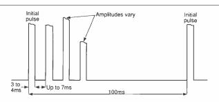
Fig. 2: Four-pulse Russian 'Woodpecker' transmission, unmodulated sequence (see text).
