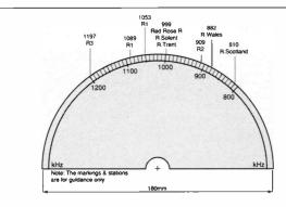
Fig. 1: How to mark out the dial.
