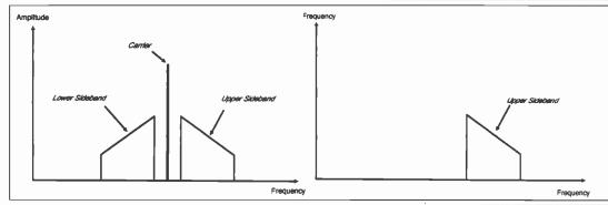
Fig. 1: An a.m. signal.
