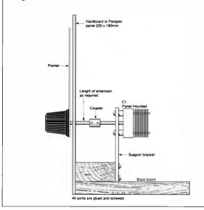
length of 1.5mm 'twin & earth' lighting cable is ideal). Place in position and wind three turns tightly round the shaft using a pair of pliers. The pointer can now be soldered or glued to the shaft.
