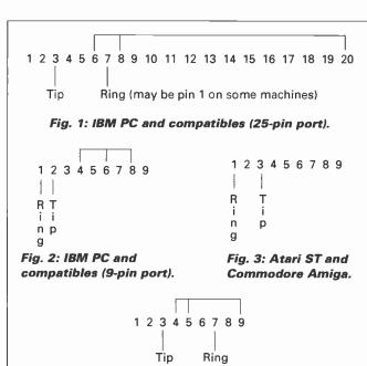
Fig. 4: ZX Spectrum with interface 1 (as yet untested).
