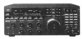
The NRD525 is a high class, general coverage receiver with expandability looking to the future. Combining traditional technology unique to JRC with the most advanced digital technology superb performance whists remaining extremely easy to use. The NRD525 covers 90kHz-34MHz and with an optional VHF/UHF converter also covers 34–60, 114–174 and 423–456MHz. Modes of operation CW, SSB (USB/LSB), AM, FM and RTTY with optional demodulator.
