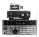
The FRG9600, a premium scanning receiver covering 60–905MHz. SSB, CW, AM & FM modes. 99 memories. 5, 10, 12.5, 25 & 100kHz scanning steps. Keyboard frequency entry. Optional convertors to extend range from 0.15–30MHz and 800–1300MHz.
