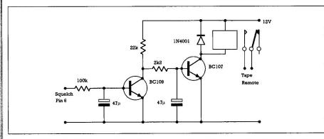
Fig. 1: Tape recorder switching from the squelch pin. The circuit also works with any receiver using the MC3357 i.f. circuit.
