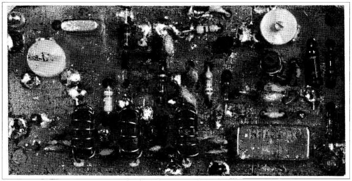
The completed prototype converter board showing the components soldered in place. Note how some components have one of their leads soldered directly to the copper earth plane which covers the component side of the printed circuit board.
