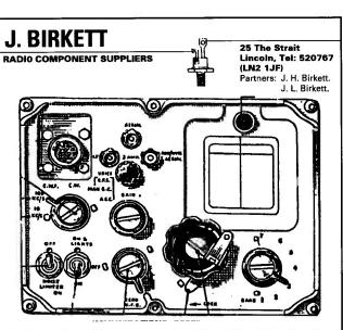
EX-MILITARY COMMUNICATIONS RECEIVER R210. Frequency 2 to 16MHz in 7 switched bands AM, CW, SSB, FCo, Aerial inputs 80ohm balanced line, long wire or whip, CW filter, BFO, Noise blanker, complete with 240 volt AC power pack, loudspeaker, headphone jack and pair of lightweight headphones.
