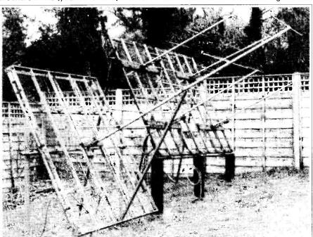
Fig. 2,3; The 136MHz array with a 95MHz antenna
