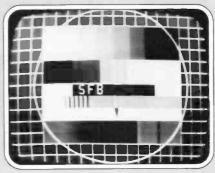
Fig. 3: The FuBK pattern is an alternative electronic test card used by many television services around the world. It was originally designed in West Germany and is now used on satellite television services.
