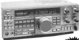
The R-5000 from Kenwood 100kHz-30MHz. SSB/AM/CW/FM/FSK
