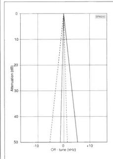
Fig. 1. Response curves of the i.f. amplifier of an Eddystone 730/4 receiver with the crystal gate switched in, and with the phasing control at maximum and minimum settings. (From Ref. 1.)
