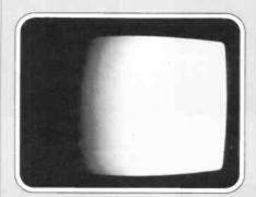
Fig. 7: The monochrome line sawtooth test pattern. This appears as a gradual change from black to white across the screen.
