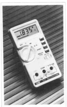
The latest instrument from TMK is a digital multimeter for all general purpose applications. Housed in a rugged, safety-yellow case, model G40 has a three-and-a-half digit, liquid crystal display with full annunciation and an analogue bar graph to indicate the movement of unstable readings. Auto ranging is supplemented by manual range selection for readings of a similar value. A reading 'hold' control and memory mode for carrying out relative measurements.
