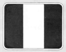
Fig. 8: This low-frequency test pattern is still radiated by a few European countries prior to the normal test card.
