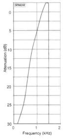
Fig. 3. Required response of a tone-correction circuit to obtain the ideal audio response for s.s.b. reception with the filter characteristics shown in Fig. 2.
