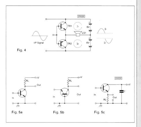
employed a complementary pair of low power (npn/pnp) transistors in the driver stage, but a matched pair of npn power transistors were operated as a single-ended push-pull output stage in Class B. When very high power levels of audio are required it may still be necessary to construct the amplifier along those lines:
