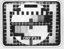
Fig. 2: The electronically-generated test card produced by Philips and known as the PM5544. When radiated with a digital clock insert it is referred to as the PM5534. This particular example is used in Austria.
