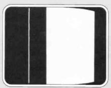
Fig. 10: The basic pulse and bar test pattern. Many European countries still use variations of this during the early stages of a test transmission.
