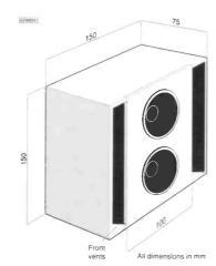
Fig. 8. Suggested loudspeaker enclosure design to provide tone correction. Note the side vents to reduce low-frequency response by cancellation. The whole front of the enclosure could be covered with a light speaker cloth.
