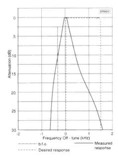
Fig. 2. Measured i.f. response of an Eddystone 730/4 receiver with the crystal gate switched in and the phasing control in the position for u.s.b. reception. The dashed curve shows the ideal frequency reponse for selective s.s.b. reception with the b.f.o. at the frequency indicated.
