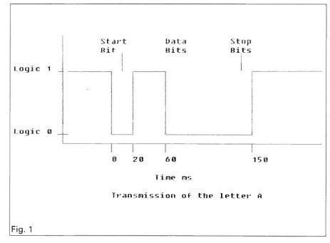
that they all stay in the right order, so that we can reverse the process at the other end. So this is the basis of serial data. Before we move on I ought make one point clear about the ITA2 code. Although I have talked about computers operating with eight bit binary numbers, the ITA2 code is actually a five bit code. This might seem a little confusing, but really all it means is that the highest three of the eight bits used in the computer are ignored.
