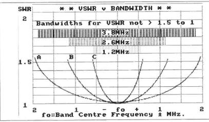
Fig. 14.1: Typical v.s.w.r. versus bandwidth of an antenna relative to centre frequency, fo.
