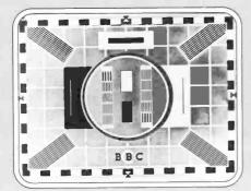
Fig. 1: The BBC Test Card 'C'. This was used by many television services around the world with minor modifications. Test Card 'C' was also used by the BBC for Regional opt-outs until the early 1970s.
