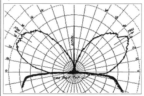
Fig.11.5: Measured pattern of vertical angle radiation from a  $5\lambda/8$  v.h.f. mobile antenna mounted on a car roof.
