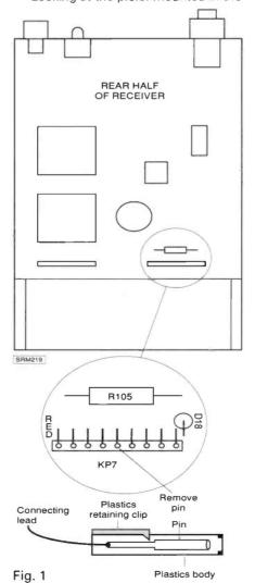
rear half of the case, locate the two white, multi-way connectors just next to the case cut-out for the battery compartment, see Fig. 1. Carefully unplug the larger of the two connectors labelled KP7. Note the connector orientation so that you can replace it later.
