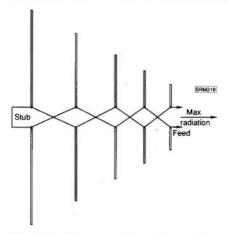
Fig.11.1: Basic configuration of the log-periodic dipole antenna; all elements are driven.
