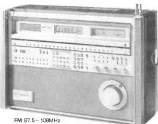
LW/MW/SW (1.6110-2.9009MHz SW (2.9010 - 30.0000MHz)
