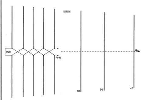
Fig.11.2: Arrangement of the log-periodic 'bandpass' antenna; D1, 2, 3 and 4 are passive elements (directors).
