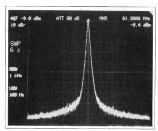
Fig. 3.2: The modified local oscillator spectrum. Scales: Horizontal 12kHz/div. Vertical 10dB/div. RX tuned to 6.15MHz; v.c.o. 61.995MHz.
