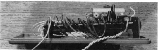
Two views of the completed Passive Signal Booster showing how it is constructed and fitted into the plastics box.
