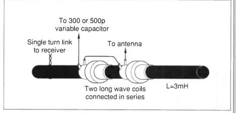
Fig. 3: Coil winding details for the l.w. version of the booster.
