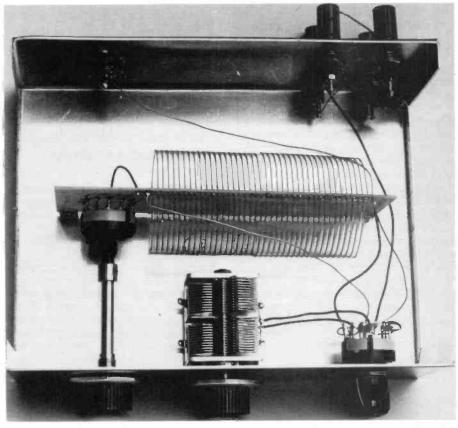
coped well with both antennas at all frequencies from 3 to 30MHz. My chief interest is the amateur bands but I used it with my general coverage receiver on all the main broadcast bands and it worked well. I also tried the TU1 with my double antenna which has a balanced twin feeder. With the balun in the circuit, it tuned every amateur band from 3.5 to 30MHz. I also used it with a low power (5 watt) transceiver on 3.5 and 14MHz and had several successful contacts on both bands.
