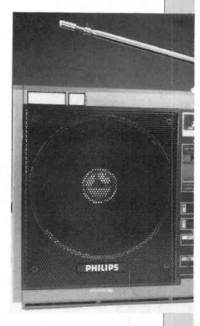
v.h.f. used 10kHz steps. One particularly useful feature was that these tuning steps automatically increased by a factor of ten when the tuning control was turned quickly. This was obviously very convenient when trying to change frequency quickly.
