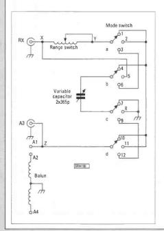
An a.t.u. is an essential part of the short wave listeners station. George Dobbs reckons that the Lake TU1 is an antenna tuning unit kit that anyone can build.
