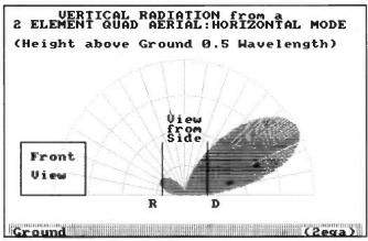
Fig. 8.3. Vertical radiation pattern for a 2-element quad at a height above ground of 0.5l.
