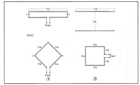
Fig. 8.1. Derivation of a quad element: "A" from a folded dipole; "B" from two driven half-wave elements spaced 0.25I apart, see text.
