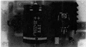
The 12V d.c. 1 amp stabilised power supply module which could also be used to power any project requiring 12V d.c.
