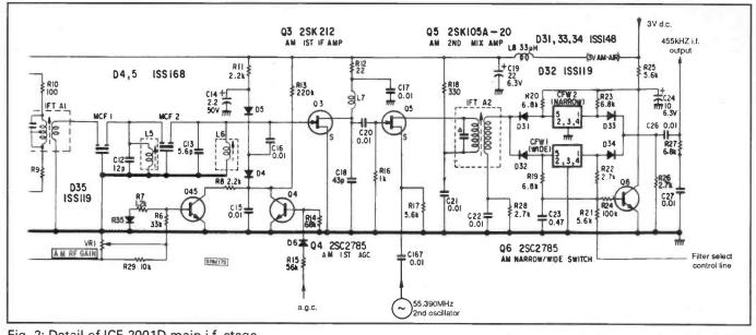
Fig. 2: Detail of ICF-2001D main i.f. stage.
