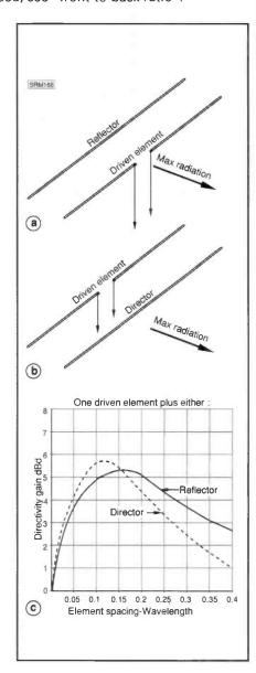
Fig. 8.5. "A" shows a 2-element quad with driven element and reflector; "B" is a 2-element quad with a driven element and director; directivity gain obtainable from either for a given element spacing is shown at "C".
