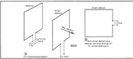
Fig. 8.2. "A" shows simple 2-element quad with driven element and parasitic reflector; "B" illustrates that horizontal polarisation is obtained by turning elements through 90 degrees.
