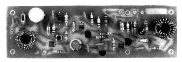
The completed 20m v.f.o. board. A dual varicap diode is fitted for tuning purposes.
