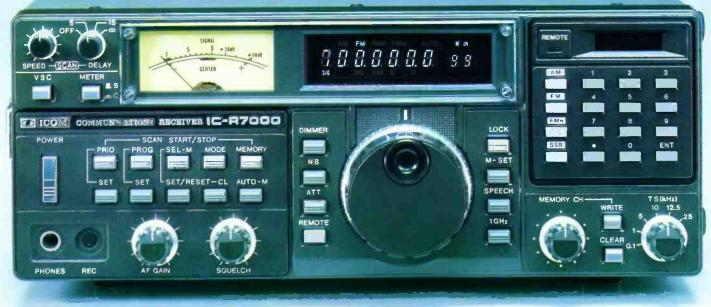
With 99 programmable memories the IC-R7000 covers aircraft, Marine, FM Broadcast, Amateur Radio, television and weather satellite bands. For simplified operation and quick tuning the IC-R7000 features direct keyboard entry. Precise frequencies can be selected by pushing the digit keys in sequence of the frequency or by turning the main tuning knob. FM wide/FM narrow/AM upper and lower ŠSB modes with six tuning speeds: 0.1, 1.0, 5, 10, 12.5, 25KHz.
