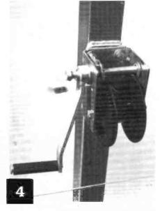
This is the DL800 Friction Braked Winch, which Tennamast recommend. It provides easier and safer control of the mast during raising and lowering. The winch is bolted onto the ground post, as shown here, using the three bolts and washers provided. The positions of the three holes means that you cannot get it upside down. The handle is wound onto the shaft and the spring and Nyloc nut fitted and tightened to retain it.
