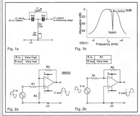
**notch depth** to be optimised, typically to -60dB below the peak i.f. response.
