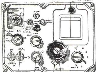
EX-MILITARY COMMUNICATIONS RECEIVER R210. Frequency 16MHz in 7 switched bands AM, CW, SSB, FCo, Aerial inputs 80 ohm balanced line, long wire or whip, CW filter, BFO, Noise blanker, complete with 240 volt AC power pack, loudspeaker, headphone jack and pair of lightweight headphones
