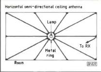
Ceiling antenna where it negotiates the lamp in the centre of the room. Note: There is no electrical connection between the lamp and antenna.
