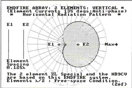
Fig. 7.2. Cardioid radiation pattern from a vertical endfire array with close-spaced elements.
