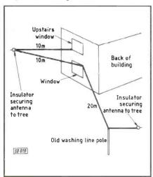
The author's dipole for 3.5 MHz bent to fit
