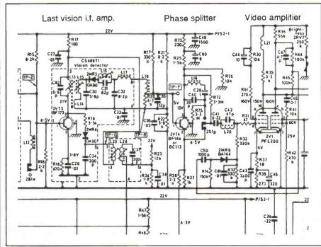
Fig. 1: Dual-standard receiver circuit (Bush TV161) with phase-splitter stage to provide positive or negative-going video.
