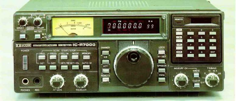
With 99 programmable memories the IC-R7000 covers aircraft, Marine, FM Broadcast, Amateur Radio, television and weather satellite bands. For simplified operation and quick tuning the IC-R7000 features direct keyboard entry. Precise frequencies can be selected by pushing the digit keys in sequence of the frequency or by turning the main tuning knob. FM wide/FM narrow/AM upper and lower SSB modes with six tuning speeds: 0.1, 1.0, 5, 10, 12.5, 25KHz.
