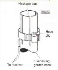
Fig. 1: Alternative jointing method
