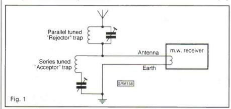
As far as m.w. reception is concerned, the best way to tackle the problem is to install a wavetrap at the receiver antenna terminal and tune it to the frequency of the interfering modulated carrier. Owing to the design of the r.f. and mixer stages some receivers are more susceptible to these effects than others - those which employ bi-polar transistors or sharp cutoff pentodes being generally inferior to those using f.e.t.s or variable-mu valves.
