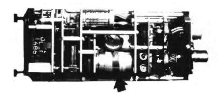
Fig. 4: The mechanism inside a servo electronic altimeter. The arrow points to a shaft encoder which supplies the radar transponder height information.
