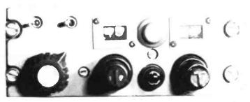
Fig. 5: Cockpit controller for a secondary surveillance radar transponder; squawking 4321 in mode C.
