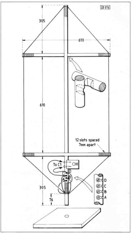
Fig. 1. Note that 14 slots will be needed in the bottom arm.
