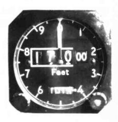
Fig. 3: QNE (1013.25mm) set. Airborne, altimeter reads FL170.
