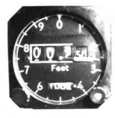
Fig. 2: QNH set to 1004mb. On the ground, altimeter reads airfild elevation of 267ft.
