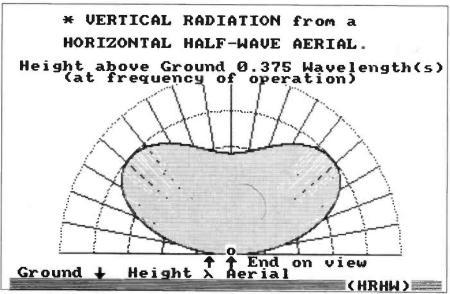
Fig. 2.6: As Fig. 2.5, but for an electrical height above ground of  $3\lambda/8$ .
