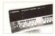
year. The models 7012 and 7013 are both fitted with temperature compensated crystal oscillators with better than 1 p.p.m. temperature stability and ageing rate per year. The case material for the 7012 is ABS plastics and aluminium for the 7013. The 7011 model costs £98 excluding VAT.
