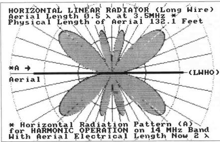
Fig. 2.3: As Fig. 2.2, but for harmonic operation at 14MHz (4 times the fundamental).
