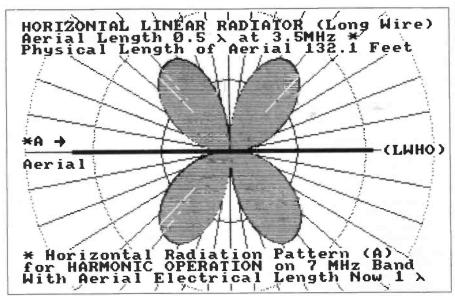
Fig. 2.2: Horizontal radiation pattern for a linear antenna operated harmonically as indicated by the annotations.
