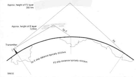
Fig. 1: Comparison of skip distance between sporadic-E and F2 layer propagation.
