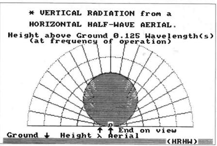
Fig. 2.5: Vertical radiation pattern for a  $\lambda/2$  antenna at an electrical height above ground of  $\lambda/8$  at operational frequency.
