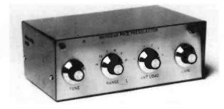
The PMX is not just another 'add on' for your receiver, not another active antenna, but something just a little bit special. It is an RF amplifier combined with an antenna tuning unit, having all the virtues of both units (normally bought as separate items) placed in one box, their circuits interlocking fully. The PMX was first designed in 1964 and although the basic idea is still the same
