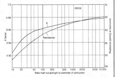
Fig. 1.2. Graph to obtain the "K" factor from the ratio of a half-wavelength to conductor-diameter; the average "K" factor is 0.95.
