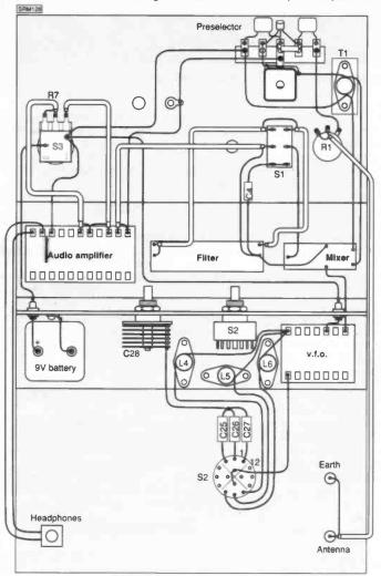
Fig. 6.1: The complete wiring diagram of the 3-Band s.s.b. Receiver. Note that the front and back panels are shown laid flat for clarity. The band selector switch, S2, has been shown removed from its correct position on the intermediate panel so that the connections to it can be shown correctly. In Fig. 5.1 the coils L4, 5 & 6 and T1 were shown incorrectly as L2, 3 & 4 and L1 respectively. These have been corrected in this drawing.
