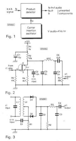
and difference products — the difference signal being the wanted audio, which is coupled to the a.f. amplifier via C5 and the gain control R3. The unwanted sum product and the reference signal are prevented from entering the audio amplifier by the r.f. choke and by-pass capacitors C3/C4 — by choosing suitable values for these capacitors, unwanted high frequency components in the audio signal can also be attenuated.
