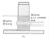
Fig. 3.4: Winding details for T1.
