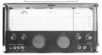
With the covers in place, connect up the receiver and run it for an hour or so with a towel covering the air vents. Keep an eye on it as the temperature will rise dramatically! If any component is likely to fail it will do so under these conditions. Switch off and allow to cool for a couple of hours, repeat the cycle and correct any faults that may have shown up.
