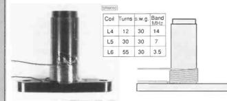
Fig. 3.3: Coil winding details.
