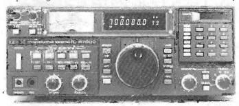
scan mode, this allows you to recall frequencies that were in use. The scanning speed is adjustable and the scanning system includes the memory selected frequency ranges or priority channels. All functions including the memory channel readout are clearly shown on a dual-colour flourescent display. Other features include dial-lock, noise blanker, attentuator, display dimmer and S meter and optional RC-12 infrared remote controller, voice synthesizer and HPI headphones.
