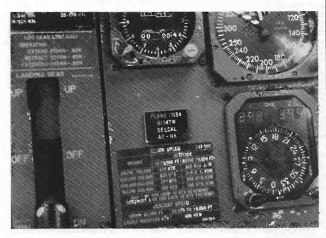
You can see the number of the aircraft and its SELCAL from the plate on the control panel.
