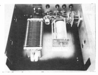
Rear panel in position. Note SWR board above variable capacitor and balun in right corner.
