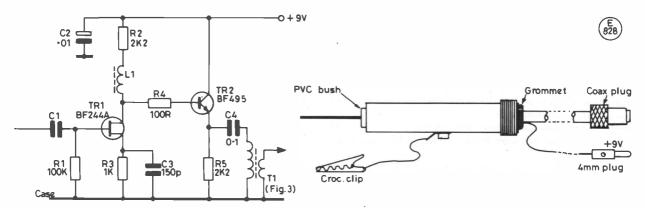
Fig. 2 PROBE CIRCUIT DIAGRAM
