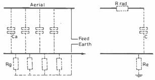
Ca Capacity between wire and earth. Rg Power wasted in ground losses.
