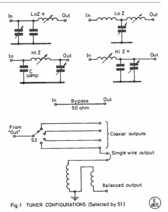
switched into circuit if required as the frequency is lowered, and more capacity is necessary to match a given load. An advantage of this type of tuner is that it always provides a two-pole low-pass response to aid harmonic rejection.
