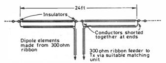
1a. Loft mounted 14-28MHz aerial used at DA1PE
