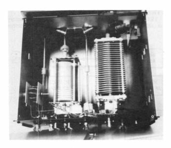
The completed ATU with top wrap-around cover removed.
