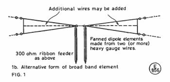
Fig. 1: (a) The loft-mounted 14-28 MHz aerial used at DA1PE consists of a simple broad-band radiating element, centre-fed with 300-ohm twin balanced ribbon feeder. Although this is used as a tuned line, losses are acceptably low because of the short indoor feeder run. The 24-ft. dipole length is set by the size of the loft.
