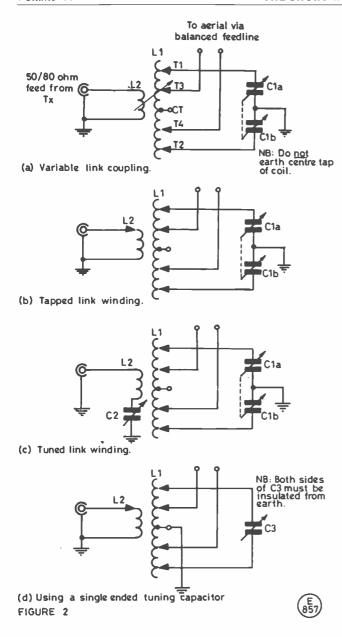
Fig. 2: The link coupled parallel-tuned matching unit for use with balanced feeders showing: (a) variable or 'swinging' link coupling; (b) a tapped link winding; (c) a tuned link winding; (d) the use of a single-ended tuning capacitor.
