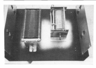
Showing assembled variable capacitor and inductor. Note the position and mounting of the side panels.
